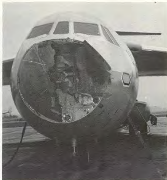
C-141 radome destroyed in encounter with hail.
