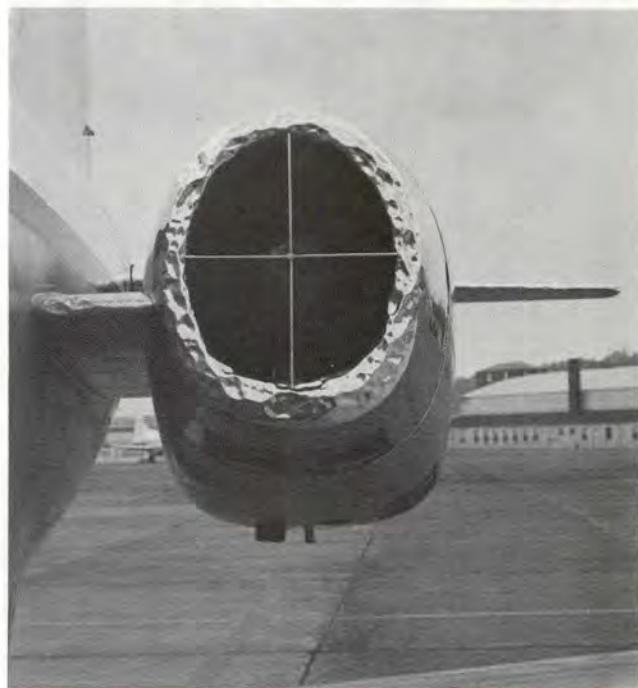
T-39 intake appears to have been attacked with a ball peen hammer. Note damage to leading edge of horizontal stabilizers.
